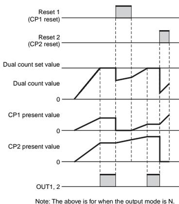
Note: The above is for when the output mode is N.
