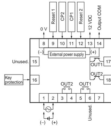
**Note:** Do not use the unused terminals for relay connections.
