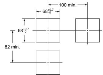
**Note:** The mounting panel thickness must be 1 to 5 mm.
