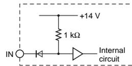
**Note:** The circuit shown above is for no-voltage input (NPN input).
