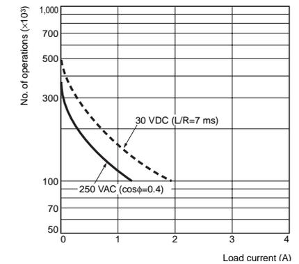
A current of 0.15 A max. can be switched at 125 VDC (cosφ = 1) and current of 0.1 A max. can be switched with L/R = 7 m/s. In both cases, a life of 100,000 operations can be expected.
