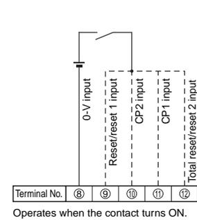
**Note:** When the H7BX is used as a tachometer, the CP2 input and total reset/reset 2 input are not used.
