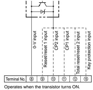
**Note:** When the H7BX is used as a tachometer, the CP2 input and total reset/reset 2 input are not used.
