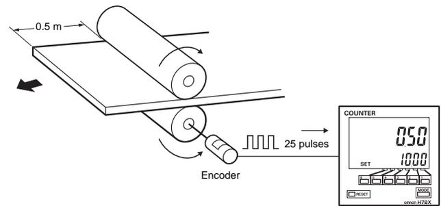
**Note:** Incorrectly setting the prescale value will result in counting errors. Check that the setting has been performed correctly before using the H7BX.
