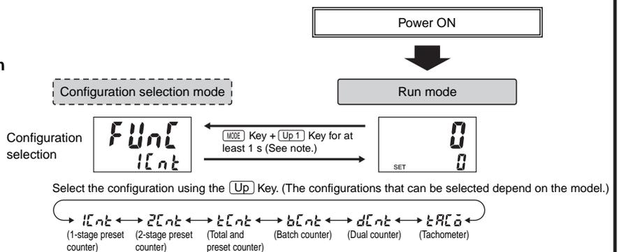
Note: This includes using a model with a 2-stage setting as a 1-stage preset counter.
