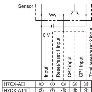
Operates when the transistor turns ON.
