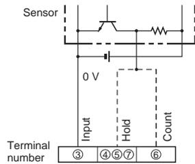
Operates when the transistor turns ON.
