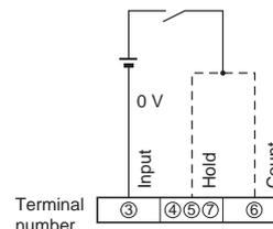
Operates when the contact turns ON.
