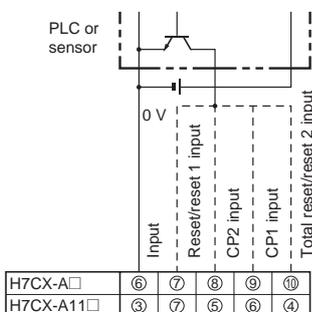
Operates when the transistor turns ON.
