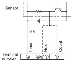
Operates when the transistor turns ON.
