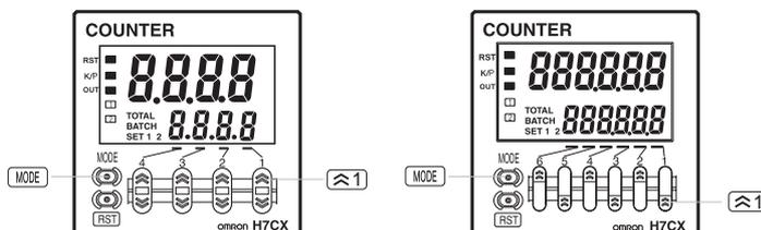
To change the mode to configuration selection mode, press the  $\approx 1$  Key for 1 s min. with the MODE key held down. The mode will not change if the  $\approx 1$  key is pressed first.
