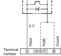
Operates when the transistor turns ON.
