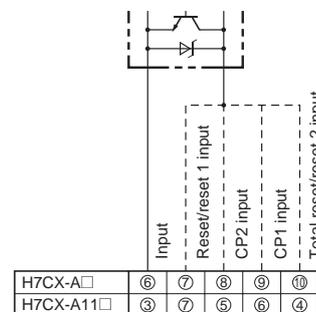
Operates when the transistor turns ON.
