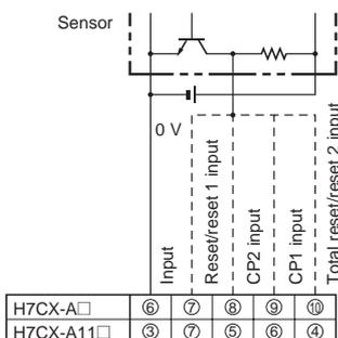
Operates when the transistor turns OFF.
