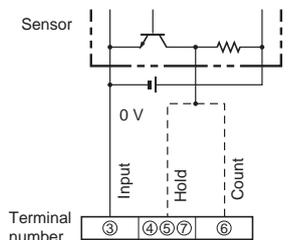
Operates when the transistor turns OFF.
