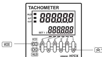
To change the mode to DIP switch monitor mode, press the **MODE** Key for 1 s min. with the **F1** key held down. The mode will not change if the **F1** key is pressed first.
