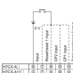
Operates when the contact turns ON.
