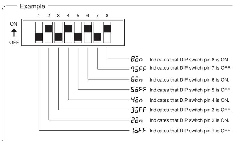
**Note:** When the mode is changed to DIP switch monitor, the measurement value is reset, outputs turns OFF, and measuring stops.
