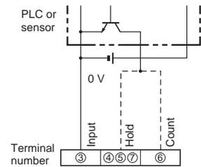
Operates when the transistor turns ON.
