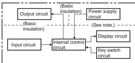
**Note:** All models except for H7CX-□D (models with 12 to 24-VDC power supplies) have basic insulation.
