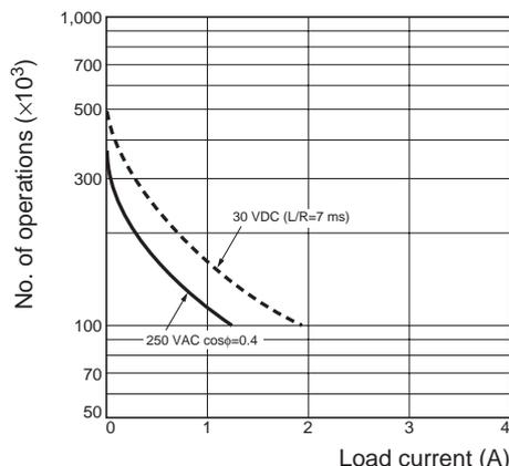
Reference: A current of 0.15 A max. can be switched at 125 VDC (cosφ=1) and current of 0.1 A max. can be switched if L/R=7 ms. In both cases, a life of 100,000 operations can be expected. The minimum applicable load is 10 mA at 5 VDC (failure level: P).
