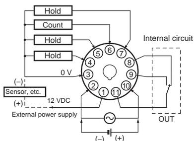
**Note: 1.** Terminals 4, 5, and 7 are all for the hold function. The function is the same whichever terminal is connected. Terminals 4, 5, and 7 are not connected internally and so do not use them for bridge wiring.
