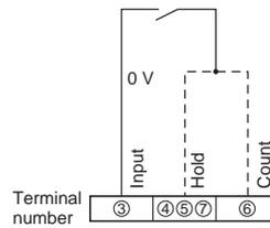
Operates when the contact turns ON.
