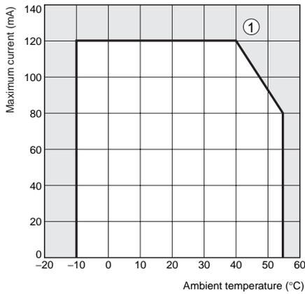
**Note:** 1. The above values were obtained under test conditions with the standard mounting. The derating curve will vary with the mounting conditions, so be sure to adjust accordingly.
