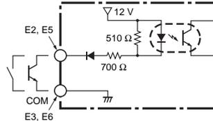
Note: A 2-wire DC sensor can also be connected. Check the ratings and characteristics tables, however, for the connection conditions.
