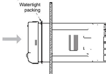
3. Insert the adaptor into the grooves on the left and right sides of the rear case and push until it reaches the panel and is fixed in place.
