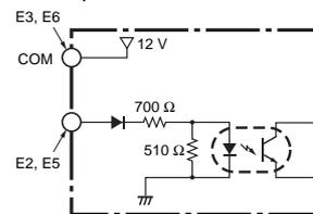
Note: A 2-wire DC sensor can also be connected. Check the ratings and characteristics tables, however, for the connection conditions.
