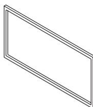
If the rubber packing is lost or damaged, it can be ordered using the following model number: K32-P1.
