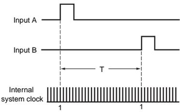
The time (T) between input A pulse and input B pulse is measured by the internal system clock. If, for example, the system clock measures 100,000 counts during time T, then
