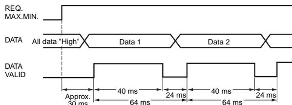
Measurement data is output every 64 ms while the REQUEST signal remains ON.
