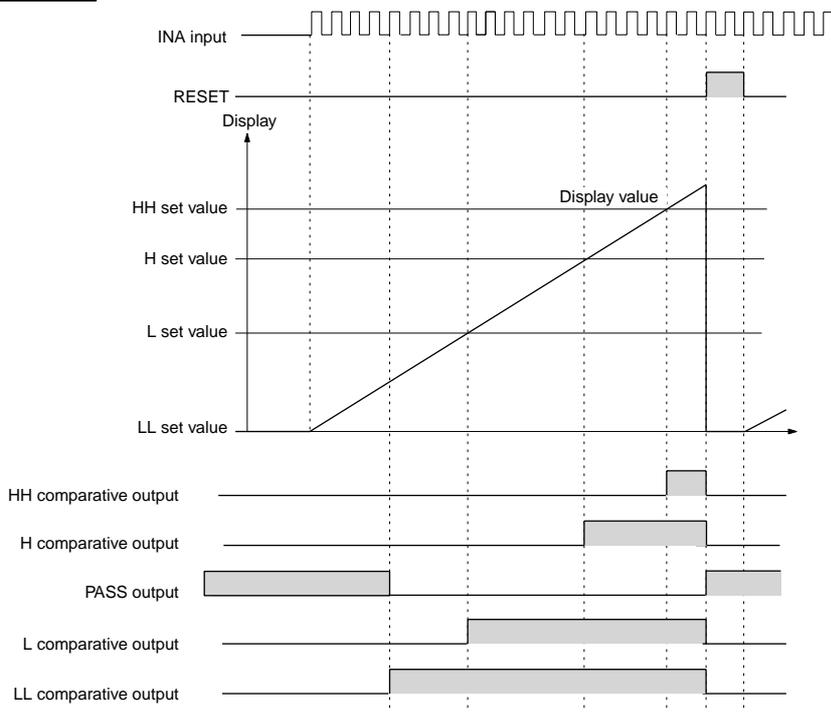
**Note:** Comparative output L or LL turns ON when the measured value exceeds the set value.
