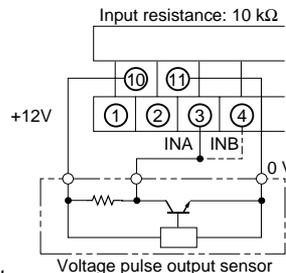
**Note:** With voltage pulse input not from a 3-wire sensor, connect the + side to terminal 3 and the - side to terminal 11.
