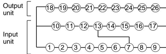
**Note:** Terminals 7 to 13 are connected internally.
