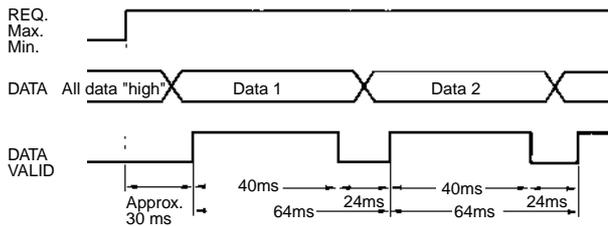
The K3NR outputs each measurement at an interval of 64 ms when a REQ signal is ON continuously.
