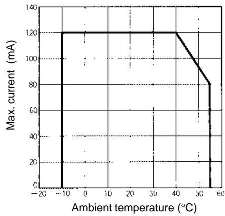
**Note:** The derating curve shown is for standard installation.
