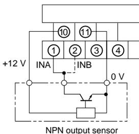
**Note:** Connect the + side of the NPN linear 2-wire input to terminal 1 and the - side to terminal 11.
