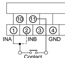
**Note:** When the contact is short-circuited, a current of approximately 13 mA will flow at a voltage of approximately 12 V.
