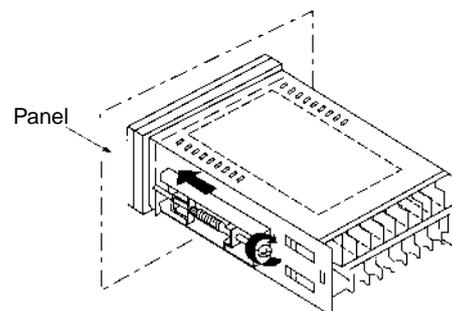
Attach the mounting bracket on the left and right sides of the Frequency/Rate Meter as shown in the illustration above and gradually tighten each screw evenly in turn by considering the balance of the tightening force until the ratchets start slipping without being further tightened.
