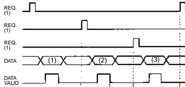
\*The period between the DATA VALID signal and the REQ signal should be no less than 20 ms max.
