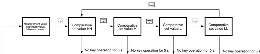
**Note:** When a comparative set value is displayed, it can be changed using the Up Key and Shift Key (if key protection is OFF).
