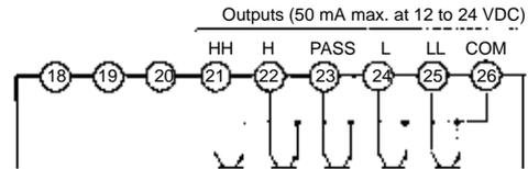
**K31-T2: Transistor (PNP Open Collector)**
