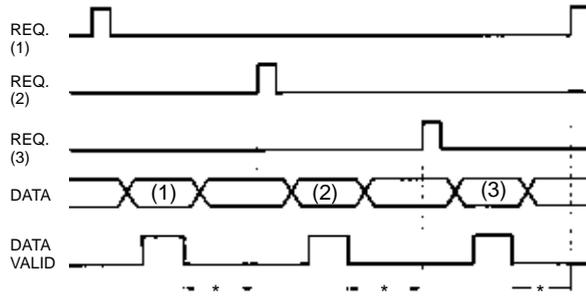
\*The period between the DATA VALID signal and the REQ signal should be no less than 20 ms max.
