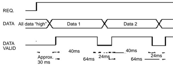
The K3NX outputs each measurement at an interval of 64 ms when a REQ signal is ON continuously.
