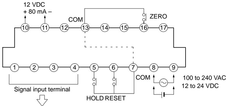
When inputting the external control signals through the open collector:
