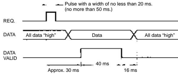
Approximately 30 ms after the REQ signal rises, a sample is taken and the DATA VALID signal is output. Read the data when the DATA VALID signal is ON.
