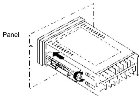
Attach the mounting bracket on the left and right sides of the Intelligent Signal Processor as shown in the illustration above and gradually tighten each screw evenly in turn by considering the balance of the tightening force until the ratchets start slipping without being further tightened.
