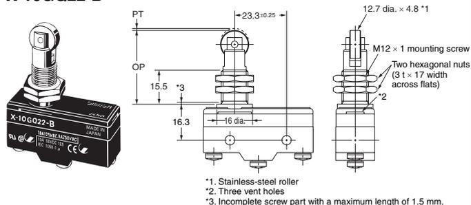
Note: Do not use both the M12 mounting screw and the mounting holes in the case at the same time. Doing so will cause stress to be applied to the Switch, possibly damaging the case or cover.
