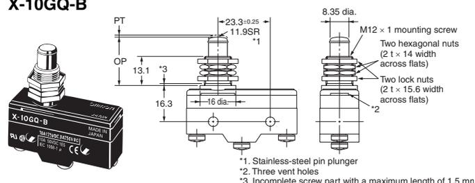
Note: Do not use both the M12 mounting screw and the mounting holes in the case at the same time. Doing so will cause stress to be applied to the Switch, possibly damaging the case or cover.
